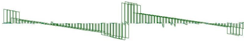
Figure 4.24 - Shear Force diagram of a composite bridge
