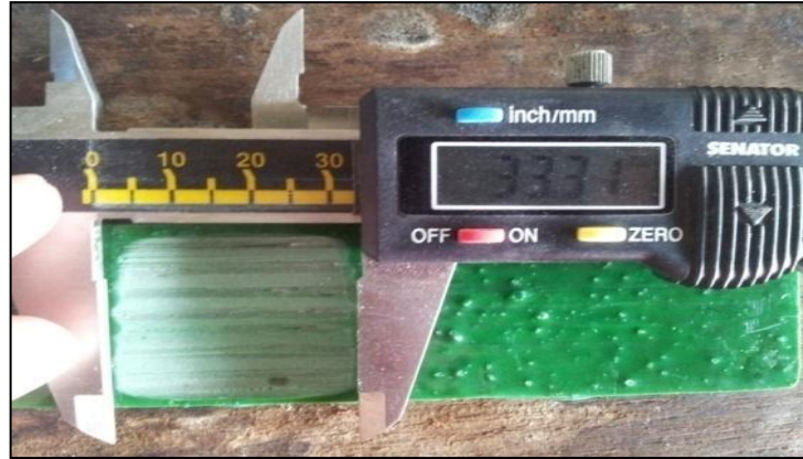
Figure 3.6.9: GFRP specimen wear scar and weigh recorded after test is conducted The GFRP specimens weight and wear scars is recorded after the test is conducted. The data then being analyses by comparing the weight loss, percentage loss and volume loss for each specimens.
