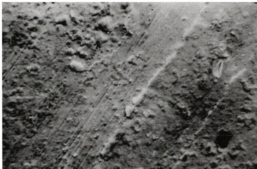
Figure 2.1.2: Wear Debris on an abraded surface
