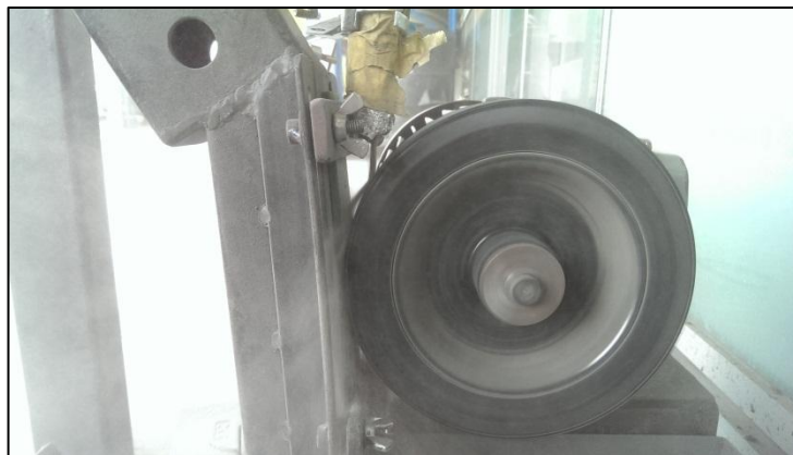
Figure 3.6.8: Wheel rubber contact with GFRP specimen
