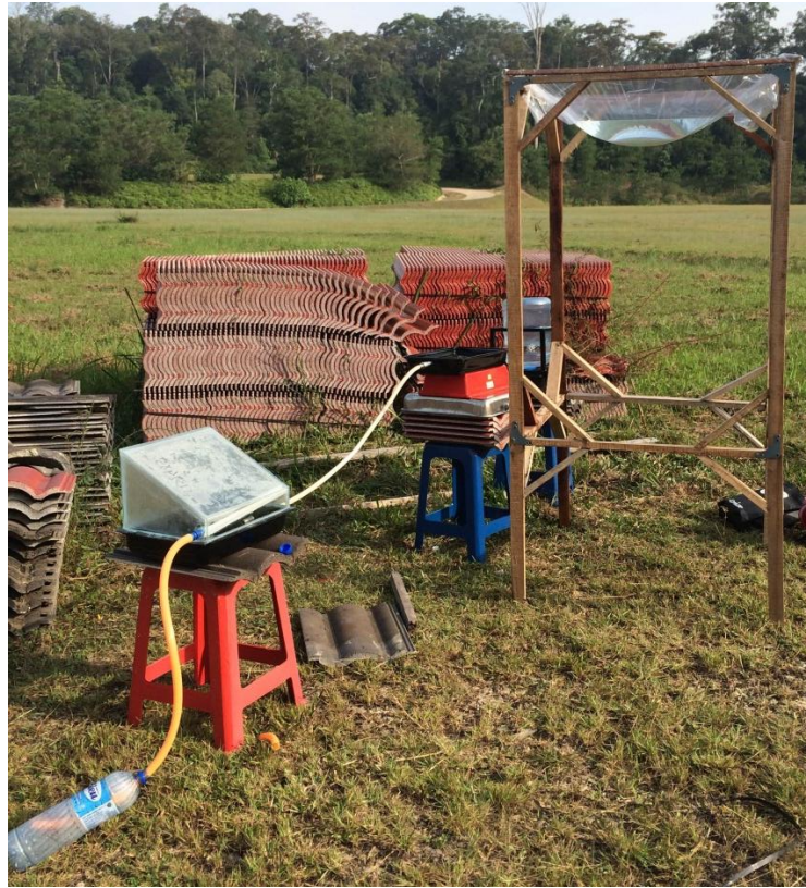
Figure 10; solar still distillation by external lens concentrator collector flow process.
