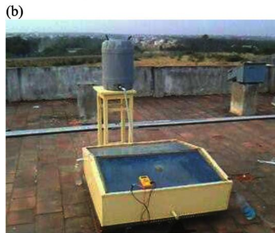
Figure 3.2: a) proposed schematic diagram of double-slope solar still b) proposed experimental still photograph
