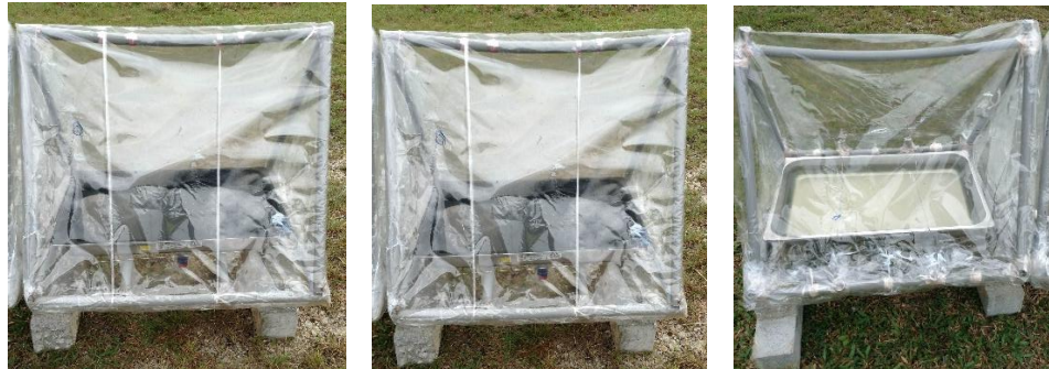
Figure 3.6: polythene film cover solar still
