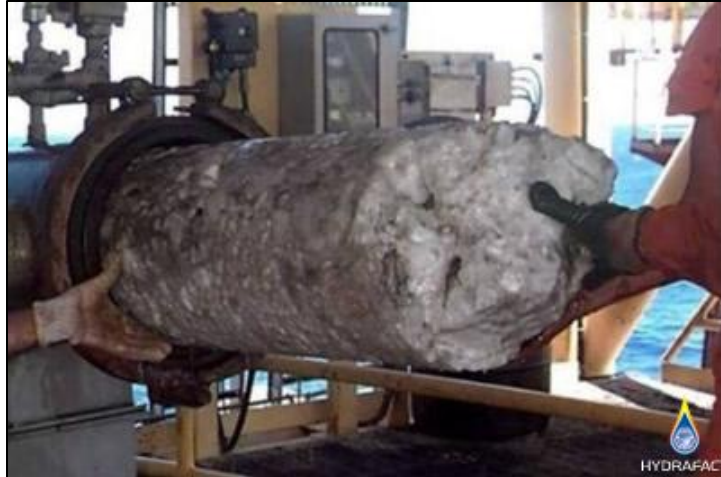
Figure 3: Gas hydrates formation in pipelines ("Gas hydrates stability,")
