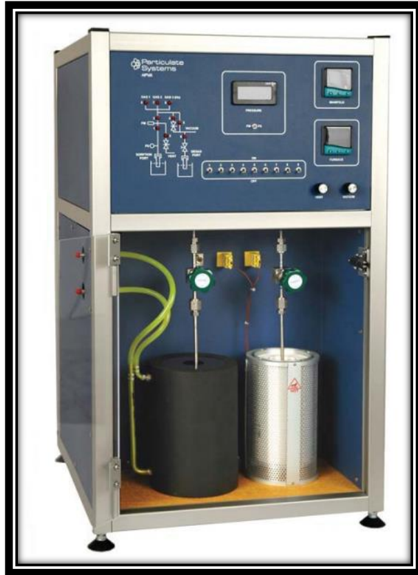
Figure 18: HPVA-II for Carbon Dioxide Adsorption Analysis
