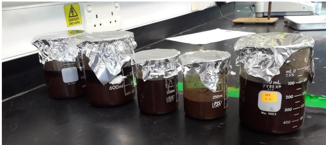
Figure 11: Banana peel powder soaked in KOH
