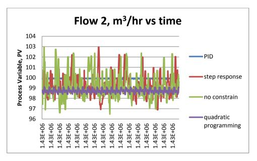
Figure 4.42: Comparison of Flow 2 controllers' response.
