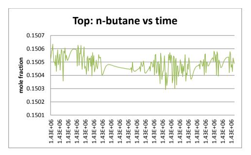
Figure 4.23: Mole fraction of n-butane at the top exit of Debutanizer.
