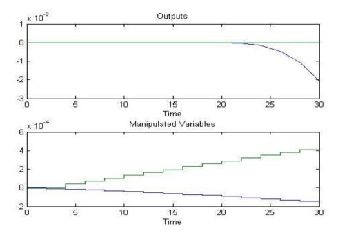
Figure 4.29: Flow 3 Controller response
