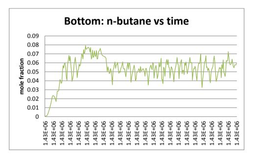
Figure 4.18: Mole fraction of n-butane at the bottom exit of Debutanizer.
