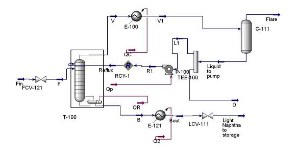
Figure 4.1: Steady State model built in HYSYS<sup>TM</sup> software
