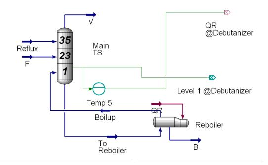
Figure 4.2: Distillation Column built in HYSYS<sup>TM</sup> software
