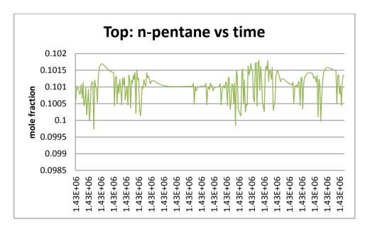
Figure 4.22: Mole fraction of n-pentane at the top exit of Debutanizer.
