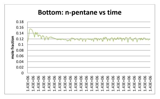
Figure 4.17: Mole fraction of n-pentane at the bottom exit of Debutanizer.
