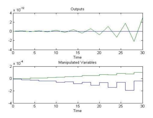
Figure 4.28: Flow 2 Controller response
