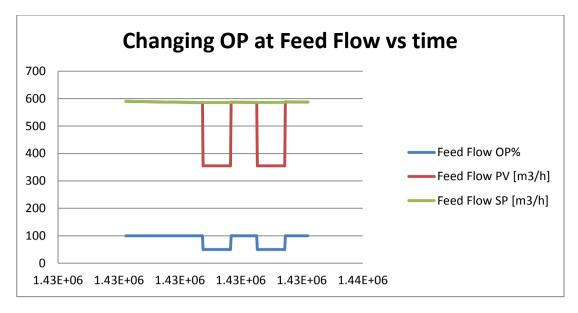
Figure 4.9: Details of Feed Flow controller during step test.
