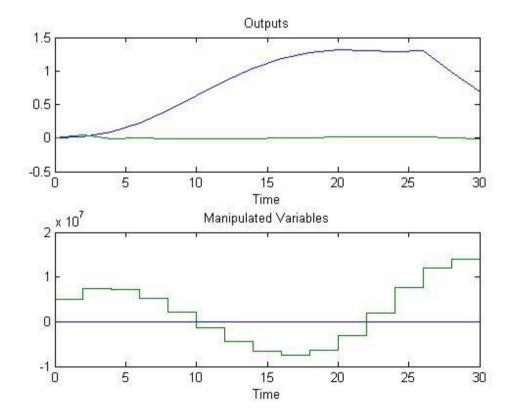
Figure 4.30: Level 1 Controller response
