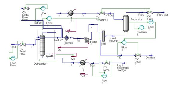
Figure 4.3: Dynamic model built in HYSYS<sup>TM</sup> software
