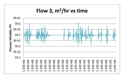
Figure 4.12: Response of Flow 3 controller during step test.
