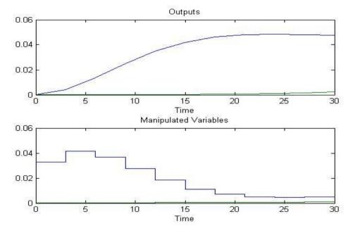
behave accordingly to the manipulated variables. A time delay is observed.
