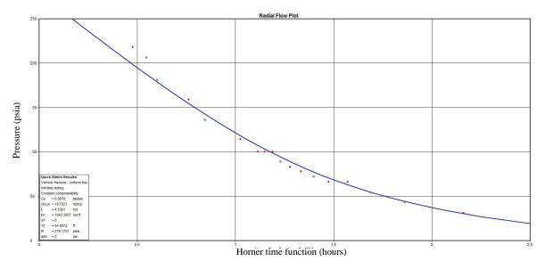
FIGURE 15. Auto Match on Radial Flow Rate Plot (Hydraulically Fractured Well)
