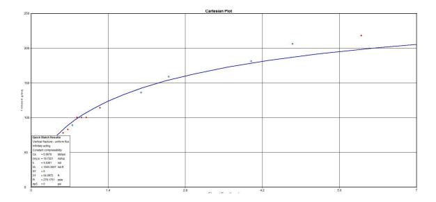
FIGURE 12. Linear Plot of Pressure Versus Time (Hydraulically Fractured Well)
