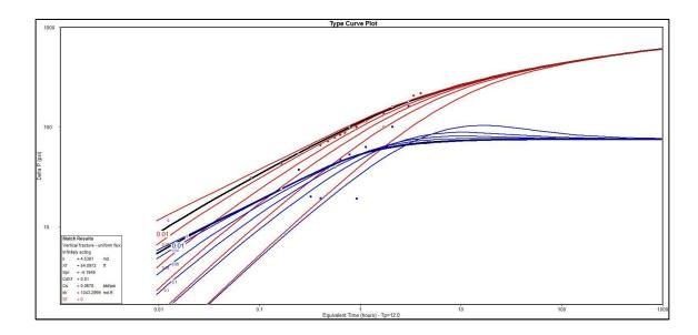
FIGURE 14. Type Curve Matching (Hydraulically Fractured Well)
