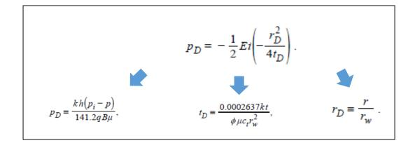
FIGURE 1. Dimensionless Parameter of Pressure, Time, and Radius That are Taken Into Account for Type Curve Analysis
