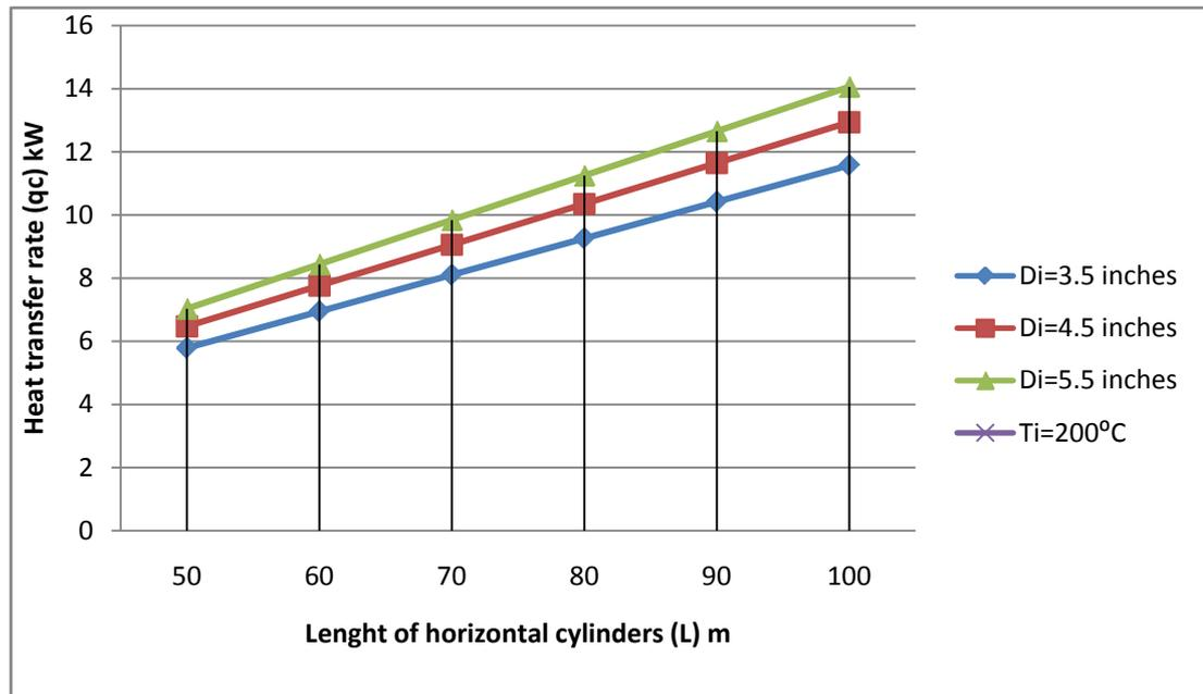
Figure 13. Heat transfer rate at different tubing diameters.
