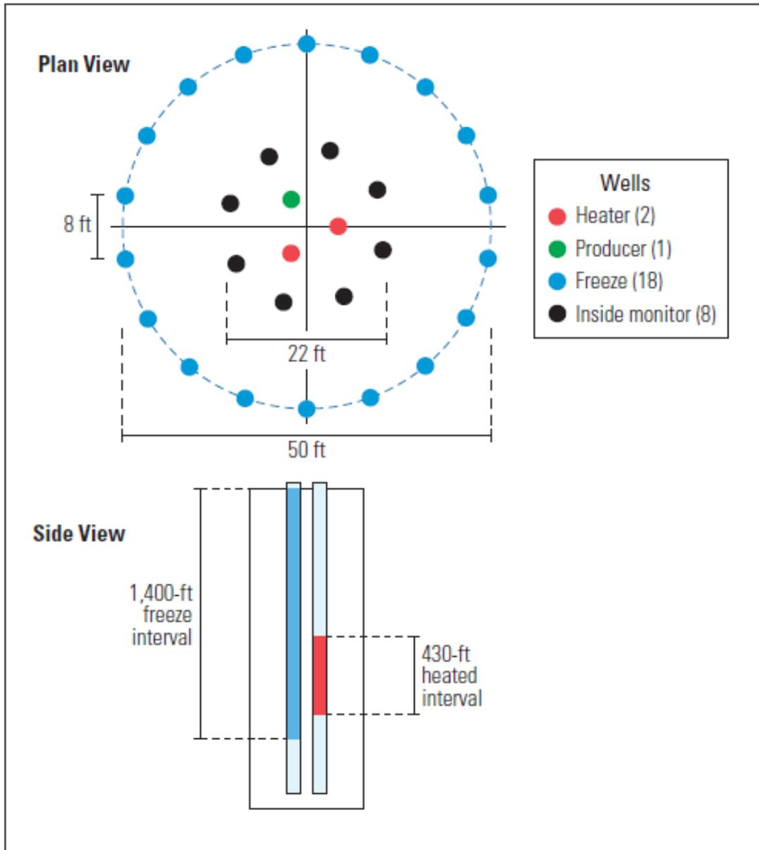
Shell ICP technology with Freezing Wall
