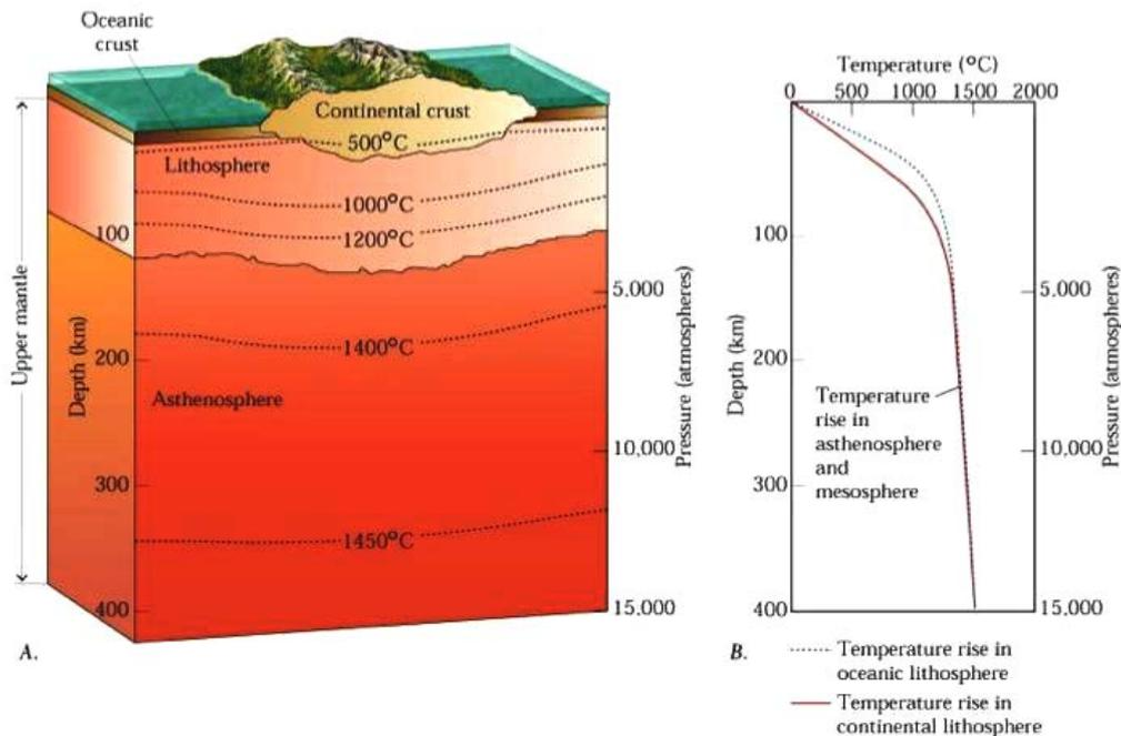
Figure 3. Earth's temperature change with change of depth (Source: Forrest, Marcucci, Scott 2007)
