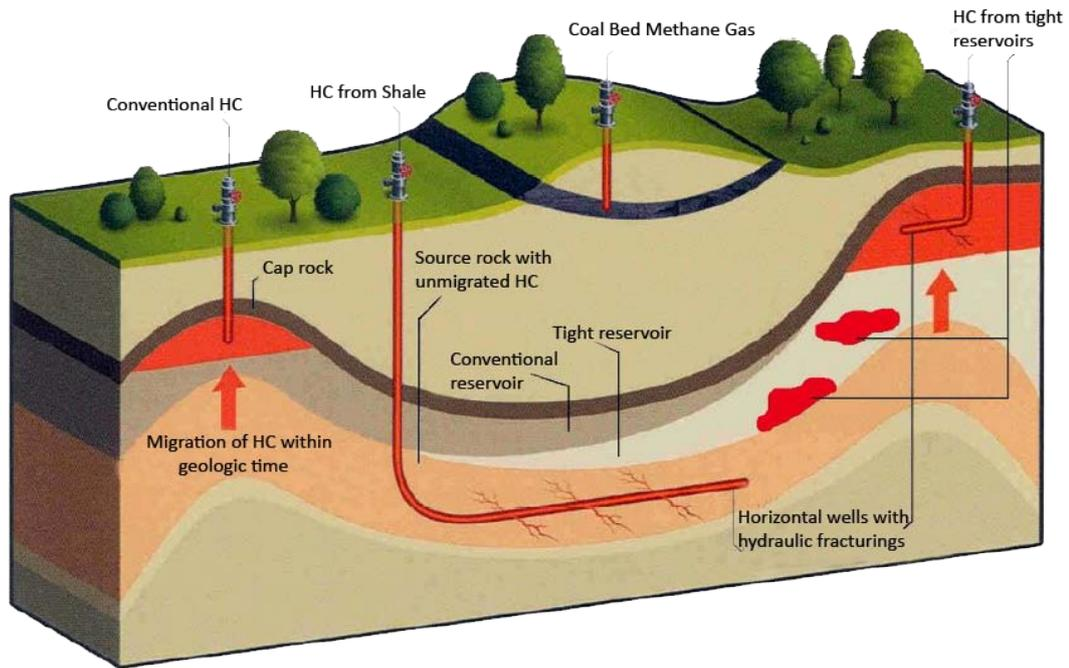
Figure 1. Types of crudes according to reservoirs (Source: Prishepa, Averyanova 2013)
