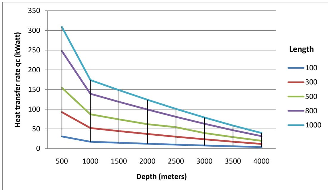
Figure 14. Heat transfer rate at varying depth of formation rock and length of horizontal section.
