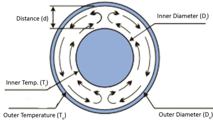
Figure 2. Free convection in annular space between horizontal concentric cylinders cross-sectional view (Source: Incropera, DeWitt, 2004)
