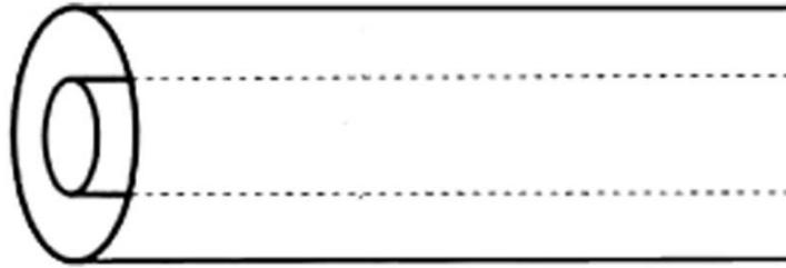
Figure 5. Casing (outer cylinder) and tubing (inner cylinder) in horizontal layout
