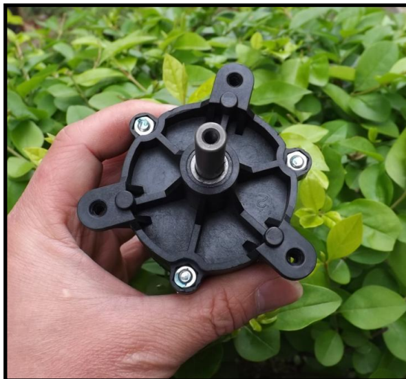
Figure 19: Generator used for the project (Top View)
