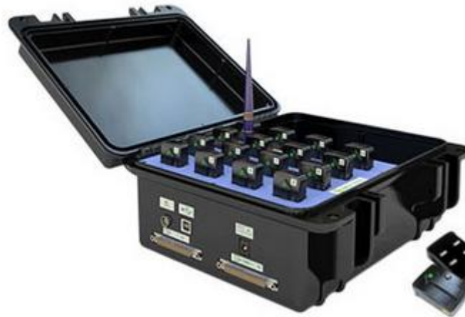
Figure 19: Delsys Wireless EMG System
