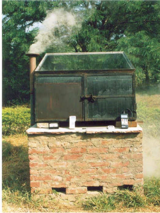
Figure 2.6: Solar- biomass hybrid drier. (Reference no. 5)
