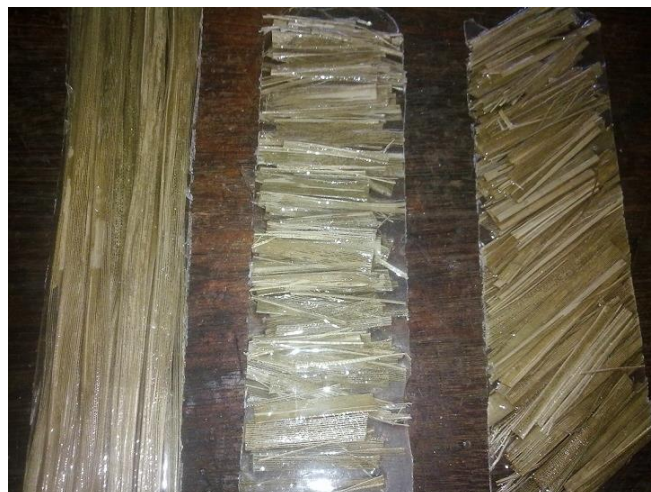
Figure 16 – Composites for mengkuang fiber of 6% NaOH concentration with different orientations
