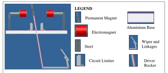
Figure 1.1: Schematic diagram of windshield wiper
