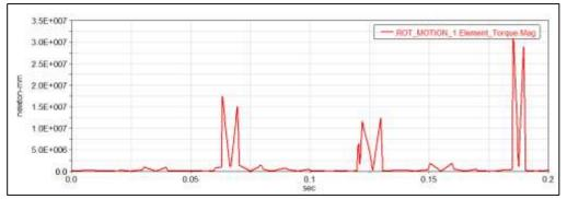
Figure 4.8: Torque magnitude at 1:0.9 ratio
