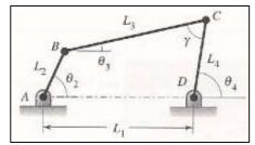
Figure 2.7: Basic four-bar linkage mechanism
