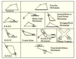
Figure 2.8: Four-bar mechanism alternative
