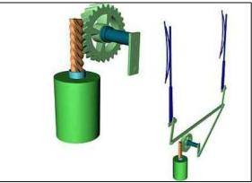
Figure 2.3: Car Wipers Working Mechanism
