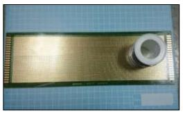
Figure 3.9: Vera Board and solder lead
