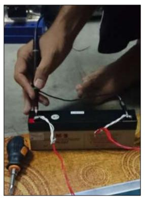
Figure 3.11: Checking Battery Voltage Value using an Oscilloscope
