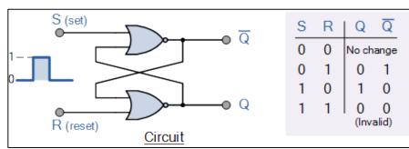
(i) one input will "SET" the device (output =1), labelled S
