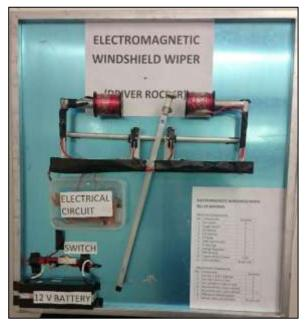
Figure 3.18: Driver rocker Assembly
