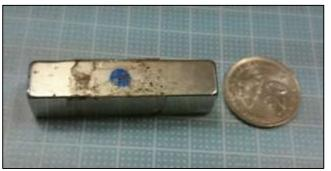
Figure 3.17: Permanent Magnet in comparison of size with 20 cent coin
