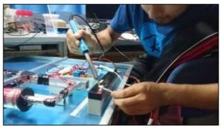
Figure 3.10: Soldering Process
