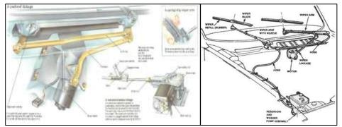
Figure 2.4: Car Wipers Linkage Mechanism
