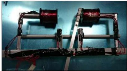
Figure 4.3: PM position with respect to electromagnet
