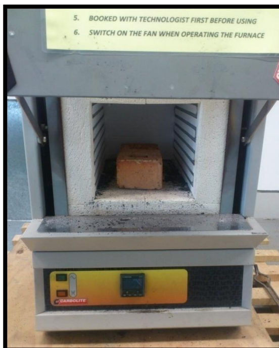
Figure 15. Heating Process (Siliconization)
