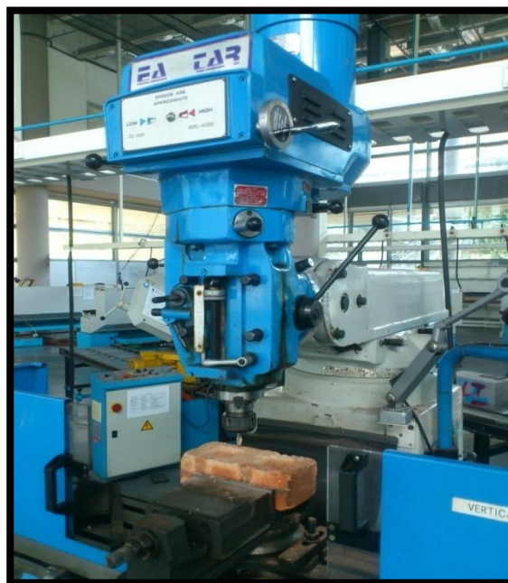
Figure 9. The brick is milled to form slots
