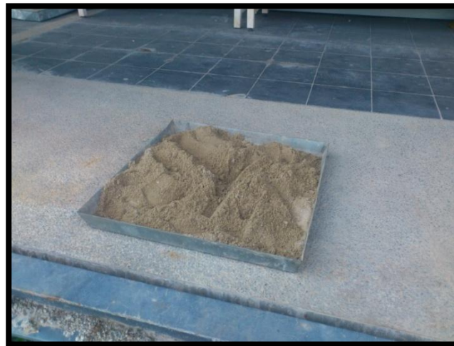
Figure 11. Sand is dried under the sun before sieving process
