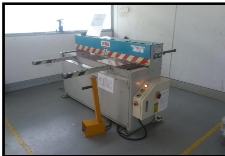
Figure 7. Process of cutting Aluminium alloy plate (Al 6061)
