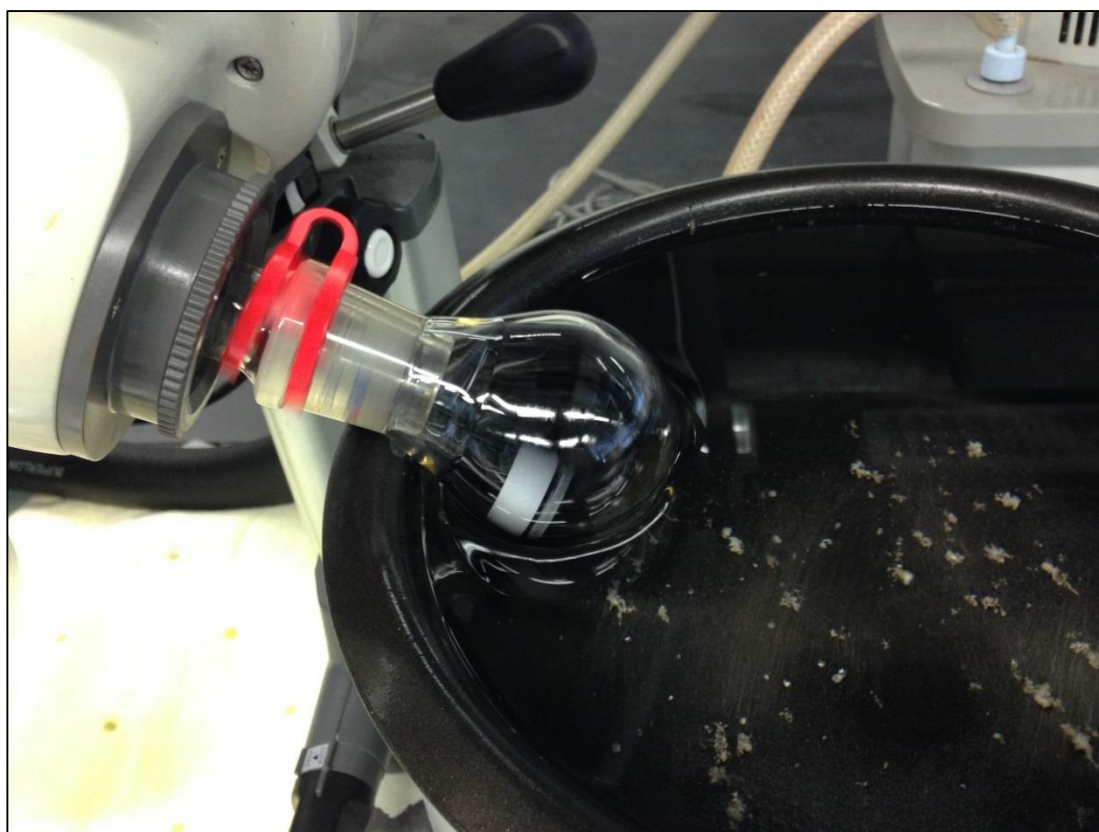
FIGURE 16: ROTAVAP Process to Evaporate the Solvent Content
