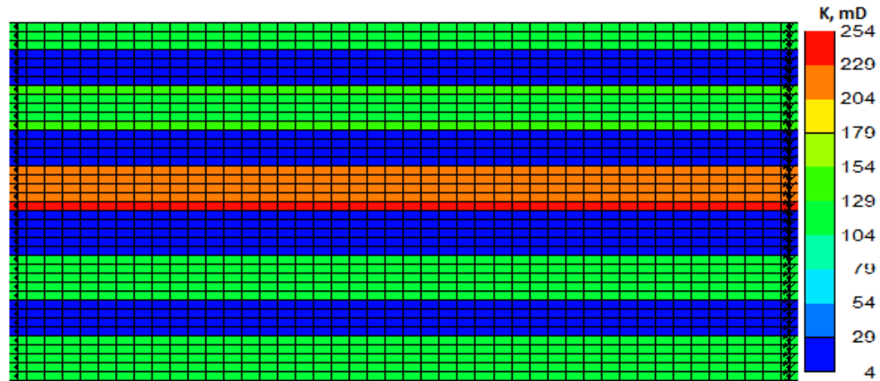
Figure 30: Permeability distribution in I-K direction
