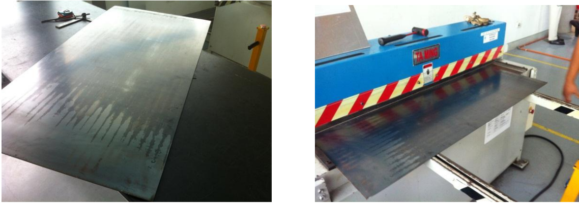
Figure 2: Cutting of steel substrate using shear cutter
