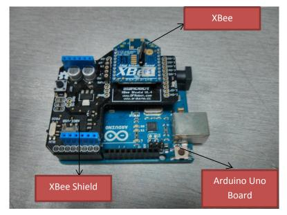
Figure 11: Modem Configuration
