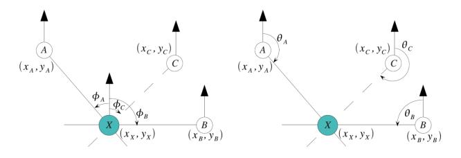
Figure 3: Angle of Arrival and Angle of Transmission [5]
