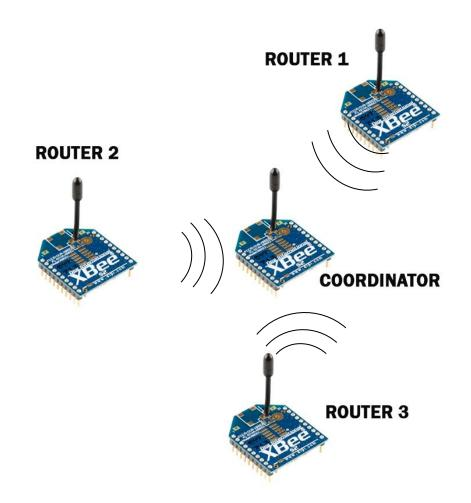
Figure 8: ZigBee Networking
