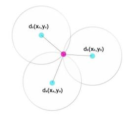
Figure 2: Intersection of three spheres in 2D using Trilateration [3]
