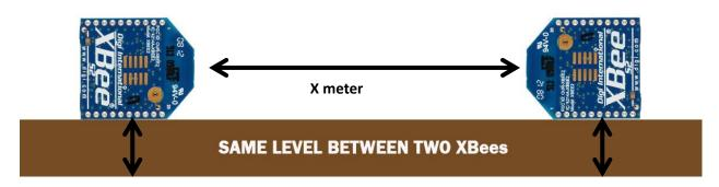
Figure 17: the XBees must be in the same level from the ground
