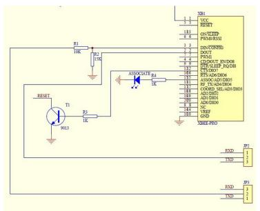
Figure 13: Schematic of XBee Shield
