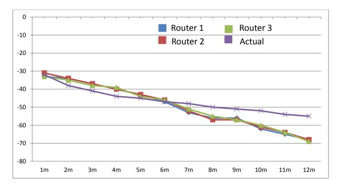
Figure 18: Relationship between Strength Signal and Distance
