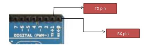
Figure 12: RX and TX pins on Arduino board
