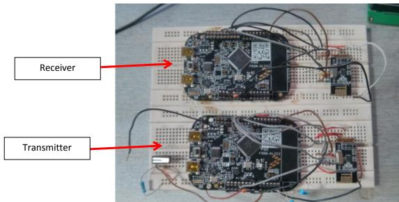
Figure 15: 2 sets of microcontroller and nRF24L01+. The top one acts as a receiver and the bottom one as a transmitter.
