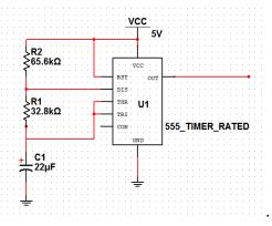
Figure 10: Timer circuit to control the Transmission duration.
