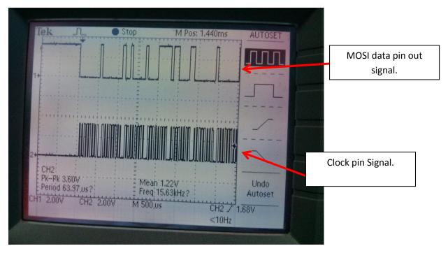
Figure41: signal captured at the clock and MOSI pin of the SPI port.
