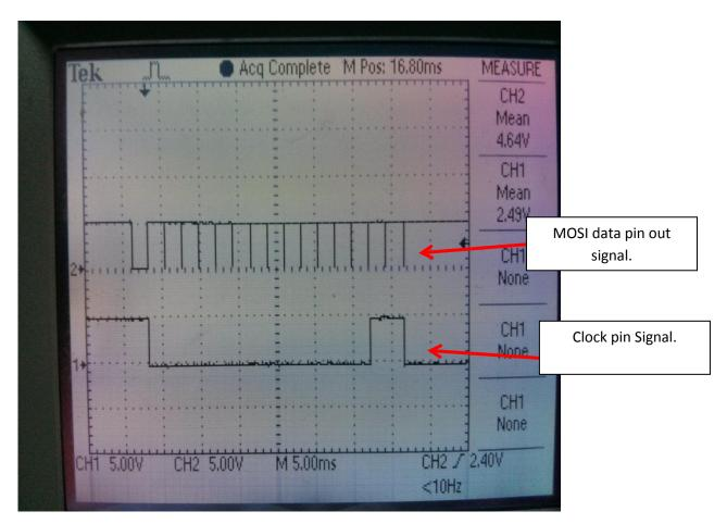
Figure 42: Timing diagram created by the code run for the test.
