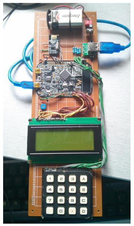
Figure 46: Hardware Prototype of the Programmer
