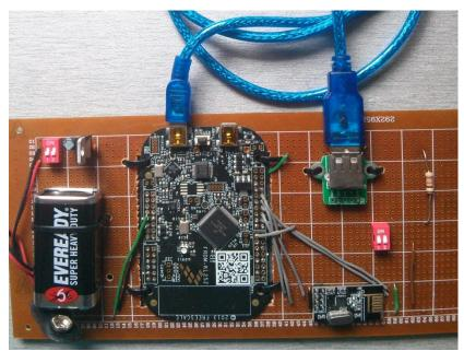
Figure 44: Hardware Prototype of Transmitter.
