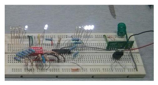
Figure 37: Receiving of 000111 binary at the receiver.
