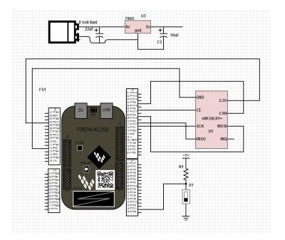
Figure 24: Schematics of Transmitter. (R1=10k).
