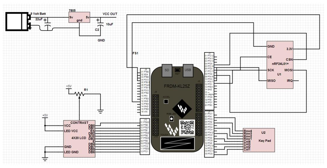
Figure 26: Schematics of Programmer.
