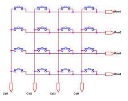
Figure23: interface connection of the keypad with MCU.
