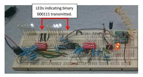
Figure 36: Transmission of 000111 binary over RF.
