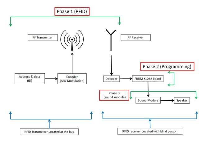
Figure 4: The overall view of the device architecture.
