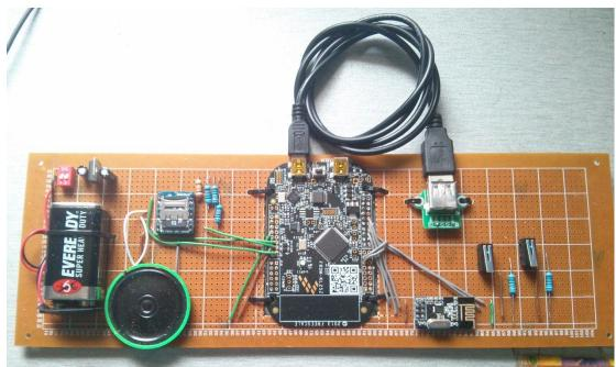
Figure 45: Hardware Prototype of the Notifier.
