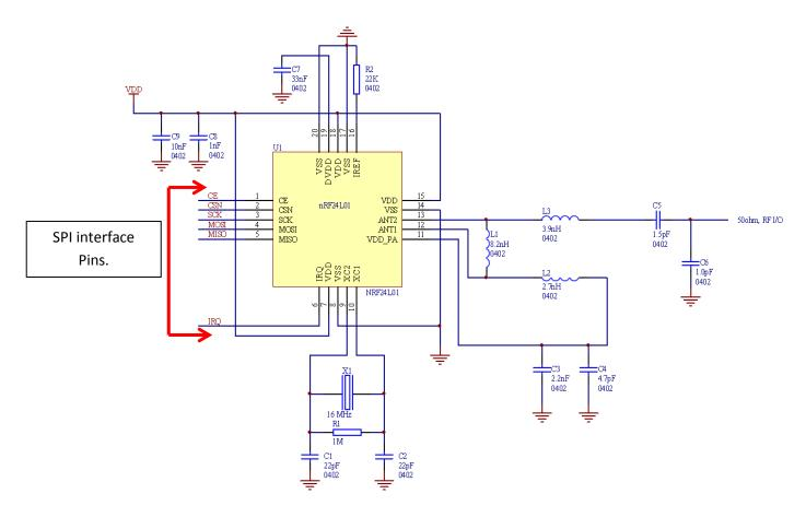
Figure 14: Schematics of nRF24L01+ module.
