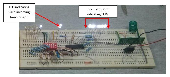
Figure 35: Actual Receiver Circuit.
