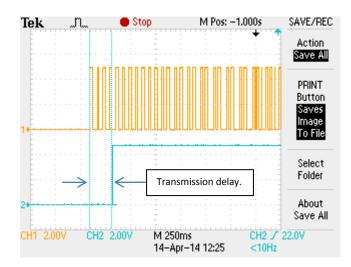
Figure 12: Transmission delay timing identification.
