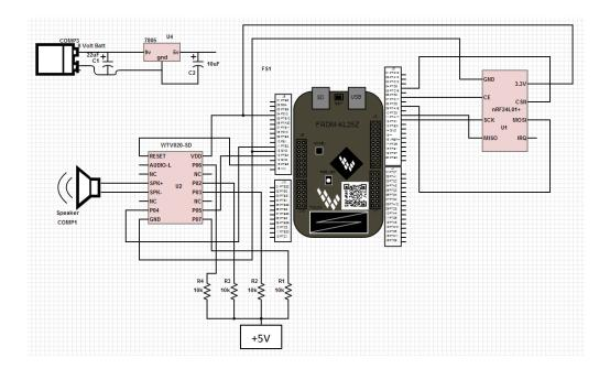
Figure 25: Schematics of Notifier.
