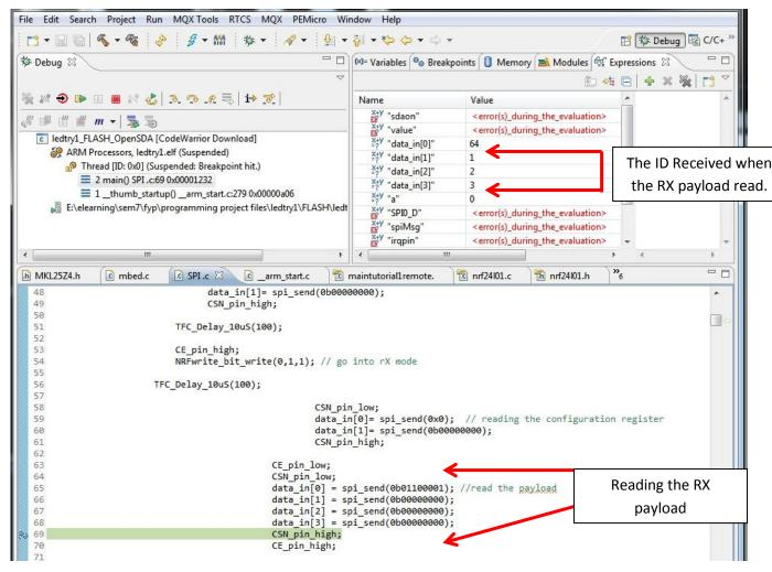
Figure 40: reading the RX payload.
