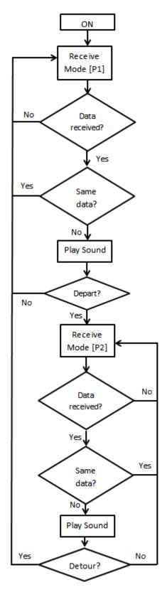
Figure 28: Firmware design of the Notifier.
