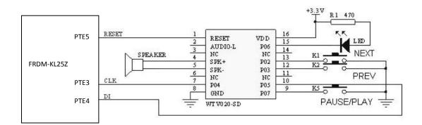
Figure 19: Application circuit diagram of sound module.
