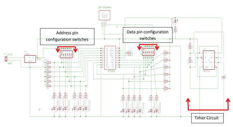
Figure 9: RFID Transmitter Test circuit.
