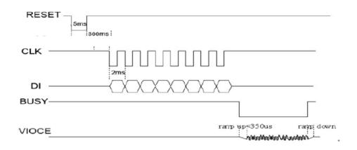
Figure 20: Timing diagram to send command to the sound module.
