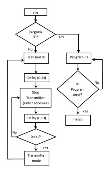
Figure 27: Firmware design of the transmitter.
