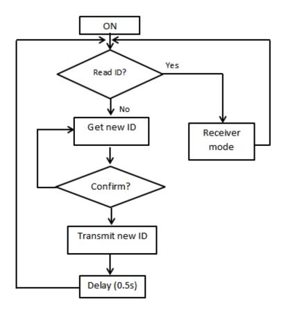
Figure 27: Firmware design of the RFID tag ID programmer.
