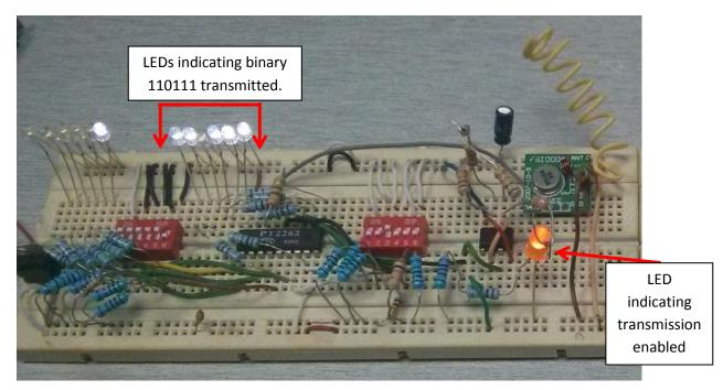
Figure 34: Actual Transmission Circuit.
