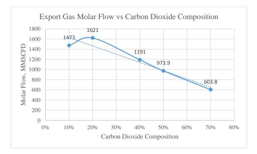
Figure 4.4-2 Graph of Export Molar Flow vs Composition of Carbon Dioxide - Case 2.
