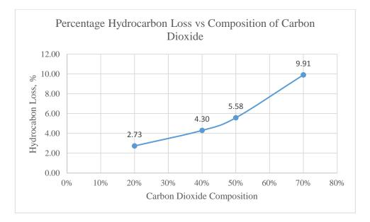
Figure 4.3-4 Graph of Percentage Hydrocarbon Loss vs Composition of Carbon Dioxide-Case 1.
