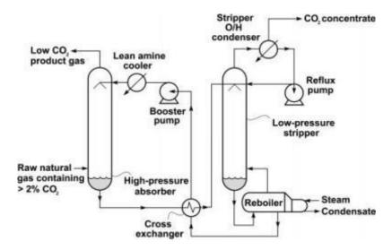
Figure 2.2-1 Typical natural gas absorber-stripper treatment process using amine absorbents (Baker & Lokhandwala, 2008)
