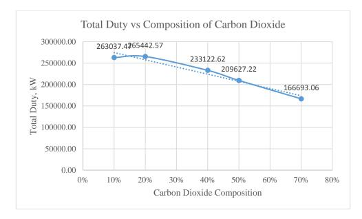
Figure 4.4-1 Graph of Total Duty vs Composition of Carbon Dioxide-Case 2.
