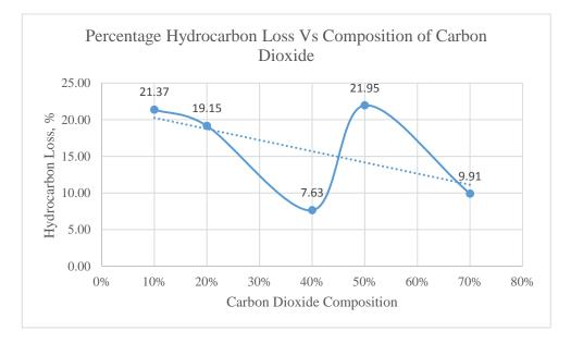
Figure 4.4-4 Graph of Percentage Hydrocarbon Loss vs Composition of Carbon Dioxide-Case 2.
