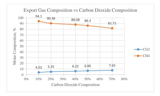
Figure 4.4-3 Graph of Methane and Carbon Dioxide Composition in Export Gas vs Composition of Carbon Dioxide-Case 2.
