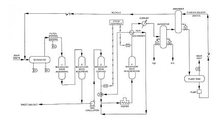
Figure 2.2-2 Closed Cycle CO2 Desorption Process Using Molecular Sieve (Mokhatab & Poe, 2012c).
