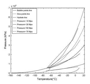
Figure 2.4-3 Phase envelope and pressure temperature distribution with the manipulated inlet stream pressure (Karimi & Abdi, 2009).
