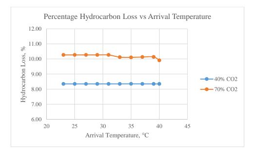
Figure 4.5-3 Graph of Percentage Hydrocarbon Loss vs Arrival Temperature.
