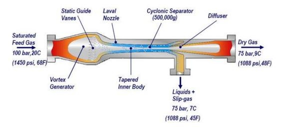
Figure 2.2-3 Cross-section view of a Gas Twister (TwisterBV, 2011).
