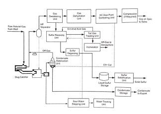
Figure 2.1-2 Typical setup of gas processing plant producing sales gas (Mokhatab & Poe, 2012b).
