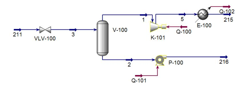
Both compressor, K-101 and pump, P-100 are not converged. This is because of the gas and liquid carry over introduced in the separator V-100. This can be ignored since the two equipment are being used to represent the recompression in Liquid Twister.
