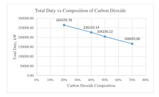
Figure 4.3-1 Graph of Total Duty vs Composition of Carbon Dioxide-Case 1.
