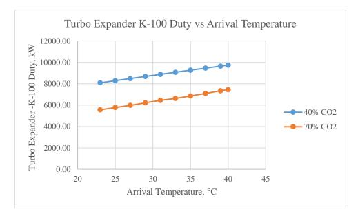
Figure 4.5-4 Graph of Turbo Expander K-100 Duty vs Arrival Temperature.
