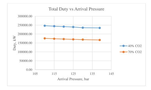
Figure 4.6-1 Graph of Total Duty vs Arrival Pressure.
