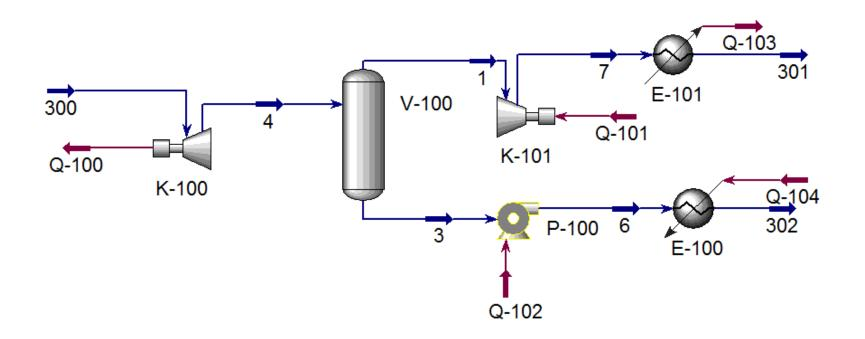
Both compressor, K-101 and pump, P-100 are not converged. This is because of the gas and liquid carry over introduced in the separator V-100. This can be ignored since the two equipment are being used to represent the recompression in Gas Twister.
