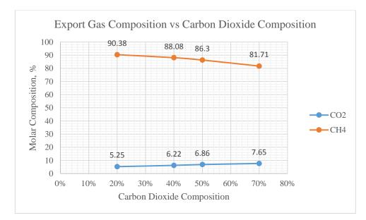
Figure 4.3-3 Graph of Methane and Carbon Dioxide Composition in Export Gas vs Composition of Carbon Dioxide-Case 1.
