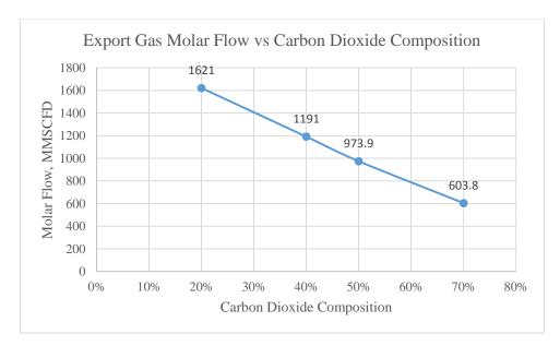
Figure 4.3-2 Graph of Export Molar Flow vs Composition of Carbon Dioxide - Case 1.
