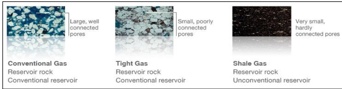
Figure 3: Types of conventional and unconventional reservoir
