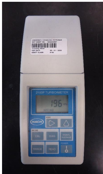
Figure 10: Measuring turbidity using Turbidimeter
