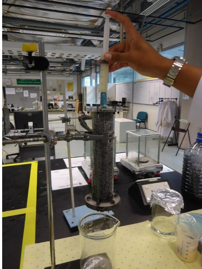
Figure 9: Injecting the formation fines solution into the sand pack
