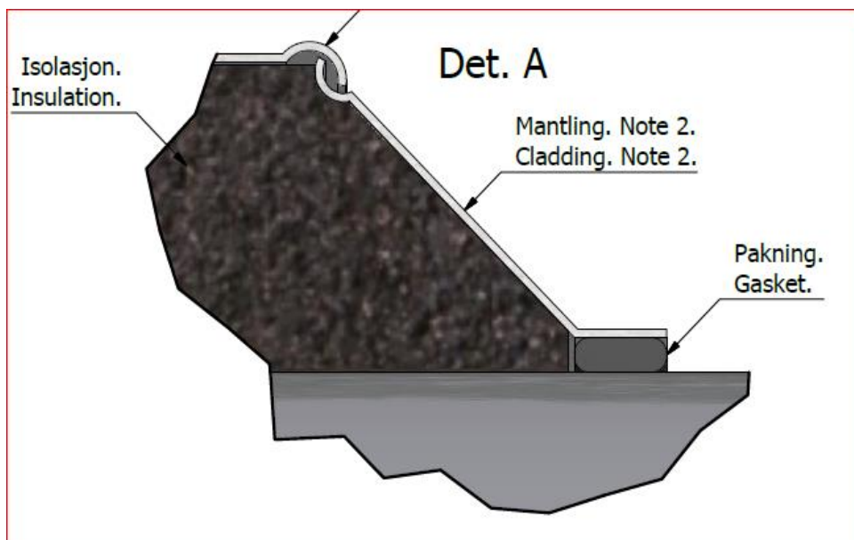
Figure 9: Focussed View of Heat Conservation Insulation of Piping
