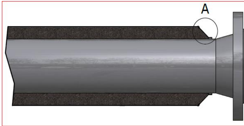
Figure 8: General View of Heat Conservation Insulation of Piping
