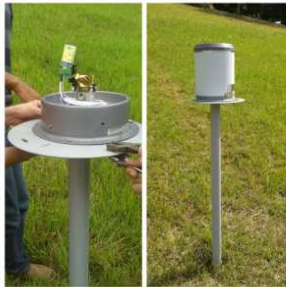
Figure 3.4: Rain gauge installed at the site
