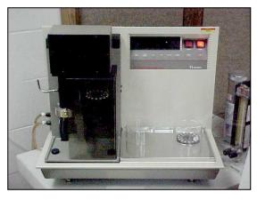
Figure 3.1: Thermal Gravimetric Analyzer (TGA) module
