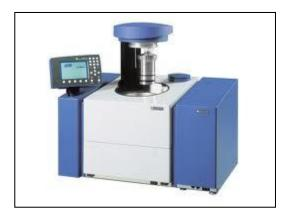
Figure 3.3: Bomb calorimeter
