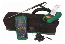
Figure 7.1: Gas Analyzer unit
