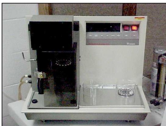
*Figure 3.1: Thermal Gravimetric Analyzer (TGA) module*
