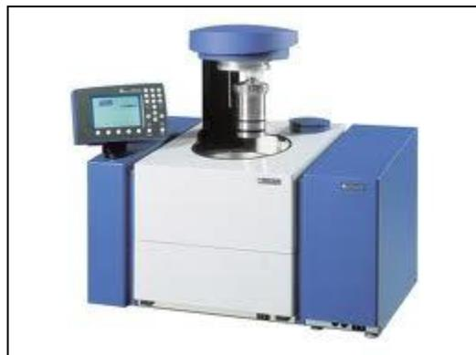
*Figure 3.3: Bomb calorimeter*
