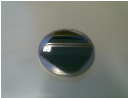
Figure 55: Polished Disc Sample
