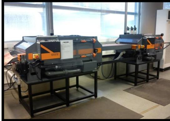
Figure 3.3.2.1 PCB Fabrication Machine
