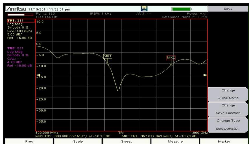
Figure 3.4.4.1 Receiver Antenna Return Loss (S11)
