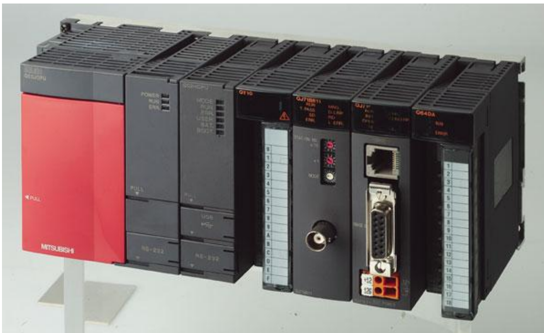
Figure 2: A programmable logic controller
