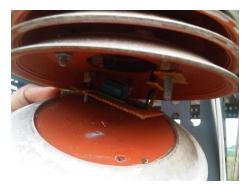
Figure 10:ambient temperature and humidity sensor
