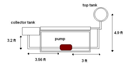
Figure 40: Solar stand pump sizing
