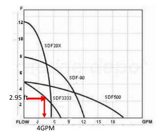
Figure 41: Pump performance chart for SDF-3333 model
