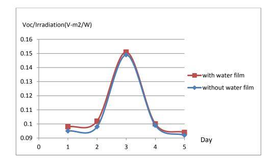
Figure 38: Comparison graph of average V<sub>oc</sub>/Irradiation for solar panel with and without water film per day.
