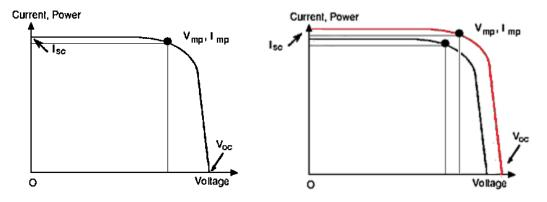
Figure 21: Isc VS Voc graph [7]. Figure 22: Increase of Vmp and Imp when Voc increases [7].
