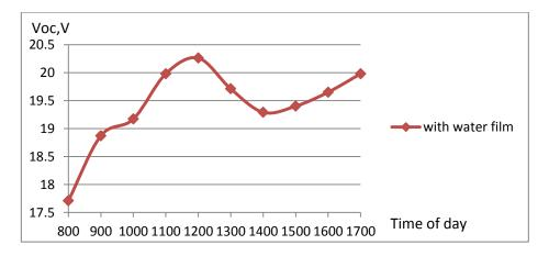
Figure 23: Solar panel with water film on 30 October 2010
