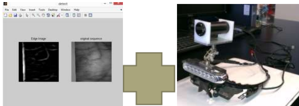
Figure 27: the combination between NIR camera and Vuzix glasses to perform real time imaging.
