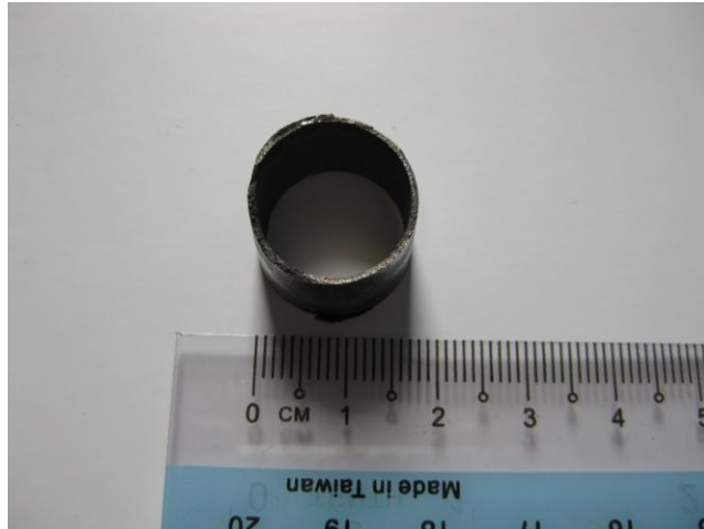
Figure 2.3: Sample material- \frac{3}{4} inch 316L stainless steel tubing.
