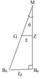
Figure 4.9: Trigonometry triangle in order to estimate the lever arm, GZ
