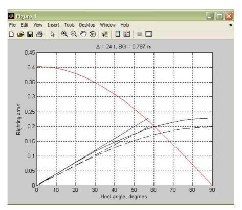
Figure 4.10: The righting arm, GZ and metacentric height, GM calculation  $[0^{\circ} < \theta < 90^{\circ}]$
