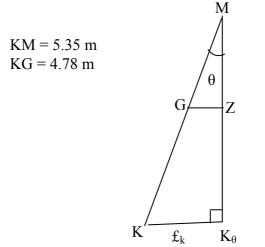
Figure 4.3: Trigonometry formed in order to find length of keel,  $\pounds_{k.}$
