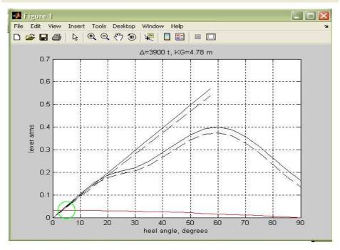
Figure 4.6: The efficient of righting-arm and metacentric height in dash line. While the red line express the heeling-arm in turning curve over the curve of statical stability.  $[0^{\circ} < \theta < 90^{\circ}]$
