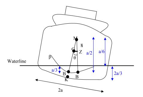
Figure 3.2: Estimate of metacentric height,  $\mu$
