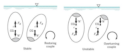
Figure 2.2: Stability of a completely immersed body – center of gravity below centroid. [1]
