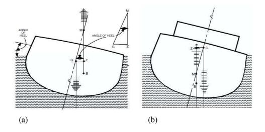
Figure 2.4: (a) Stable condition, G is below M. [5] (b) Unstable condition, G is above M. [5]
