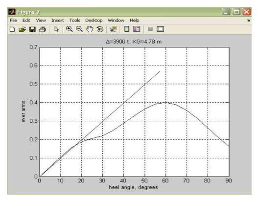
Figure 4.4: The righting arm, GZ calculation
