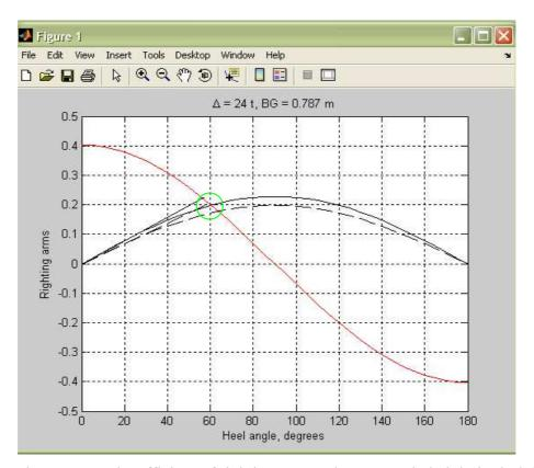
Figure 4.11: The efficient of righting-arm and metacentric height in dash line. While the red line express the heeling-arm in turning curve over the curve of statically stability.  $[0^{\circ} < \theta < 180^{\circ}]$
