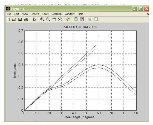
Figure 4.5: The metacentric height,GM calculation
