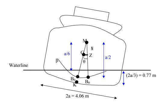
Figure 4.7: Estimate of metacentric height, GM or  $\mu$
