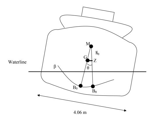
Figure 4.8: The heel angle,  $\theta$  at 10°.
