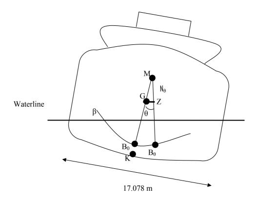
Figure 4.2: The righting couple  $10^{\circ}$  heel angle,  $\theta$ .
