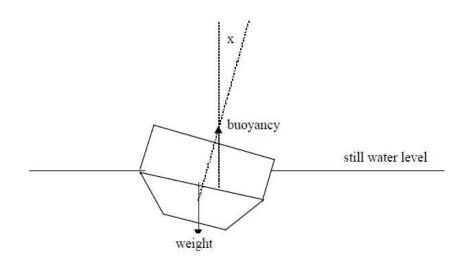
Figure 1.1: Schematic of ship in still water showing the action of buoyancy and weight to right the ship. [7]
