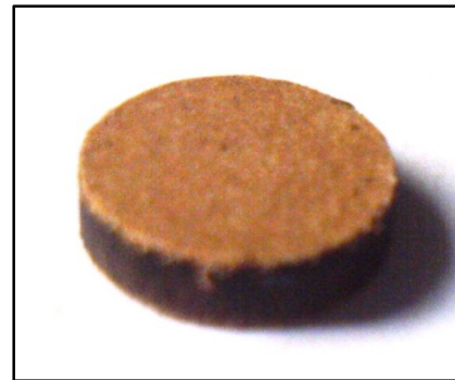
Figure 5: Sample with Suitable Compaction Force and Water Percentage
