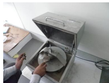
Figure 4.2 : Grinder case in inserted in the grinder machine
