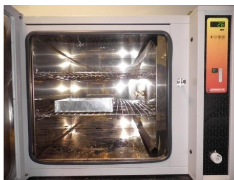
Figure 4.12 : Treated graphite is then dried in the oven at 80°C for 1 hour
