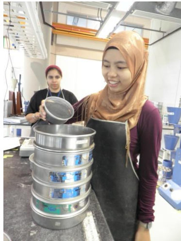
Figure 4.5: Graphite is poured into sieve
