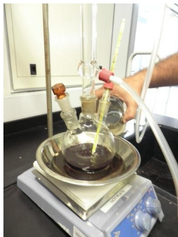
Figure 4.10 : All material is mixed well in 3 neck flask around 1 hour
