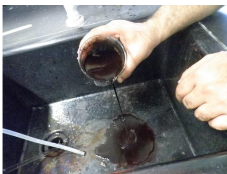
Figure 4.11 : After 1 hour, the treated graphite is washed by using distilled water until colorless
