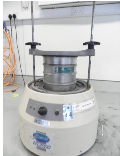
Figure 4.6: Seiver is inserted into the sieve machine
