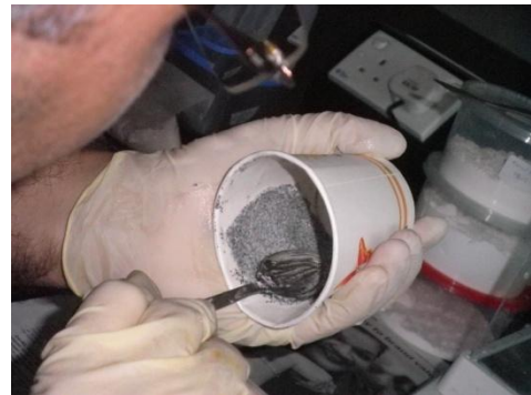
Figure 4.14 : All material is mix well by using mixer and spatula
