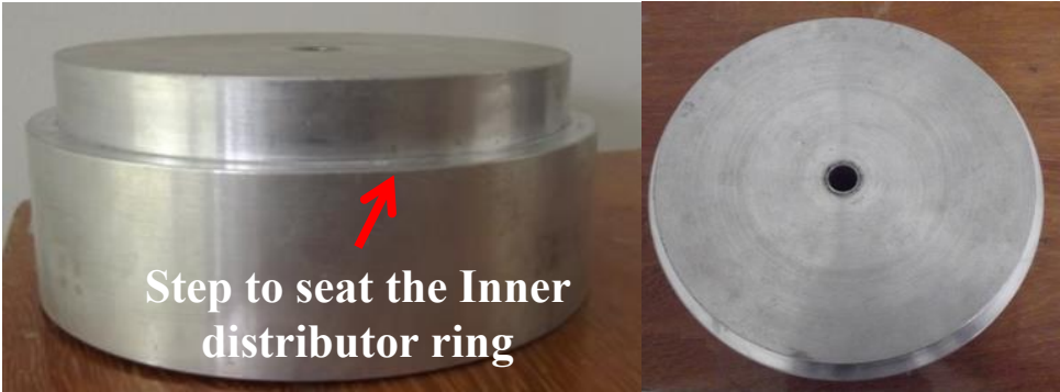
Figure 3.13: Central hub of annular spiral distributor realized
