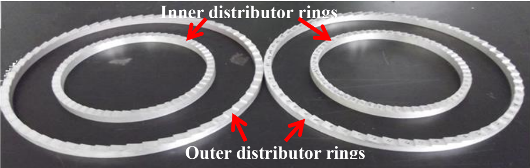
Figure 3.12: Outer and inner rings of annular spiral distributor realized
