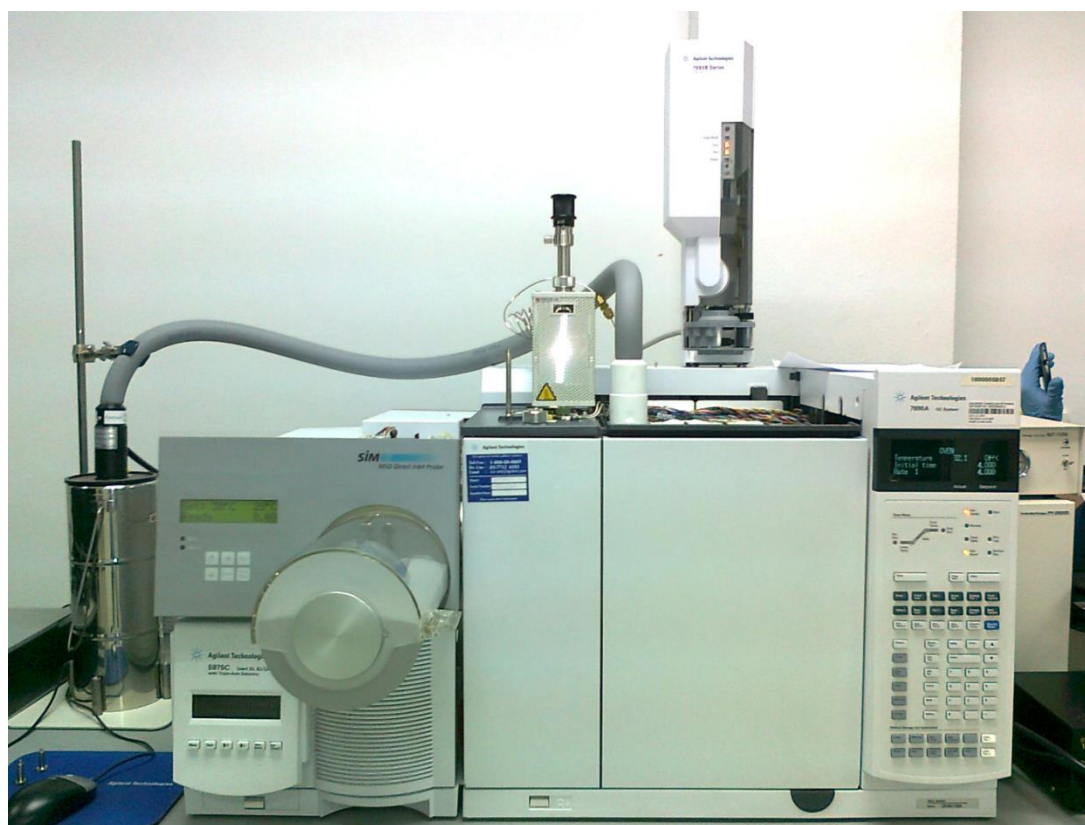
Figure 3.9: The GC 7890A” and Mass Spectroscopy with the series of “5975” produced by Agilent Technologies
