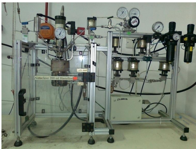
Figure 3.5: Autoclave reactor which is located in COMBICAT University Malaya (A - general view)
