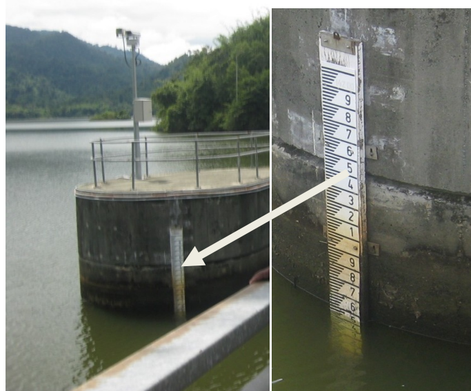
Figure 3.1 Stage measurement using a staff gage at Bersia reservoir, Malaysia
