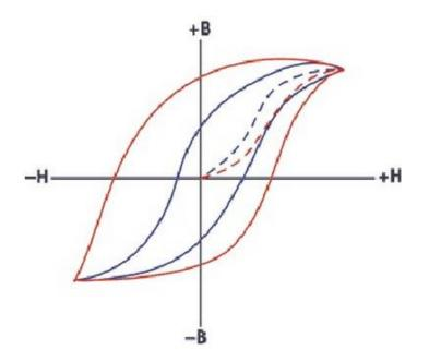
Figure 8: Hysteresis Loop (Iron VS Permalloy)
