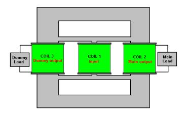
Figure 4 Bi Toroid Transformer Operating Principle
