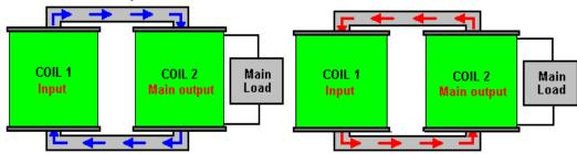
Figure 1 Conventional Transformer pulse movements
