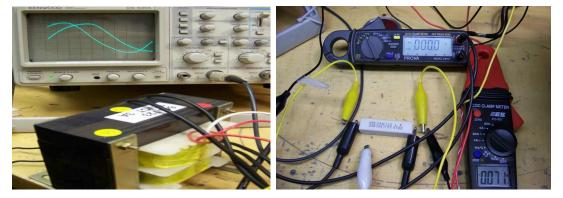
Figure 16 No Load Test
