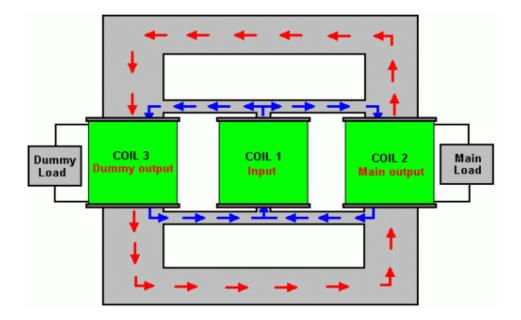
Figure 5 Bi Toroid Operating Principle
