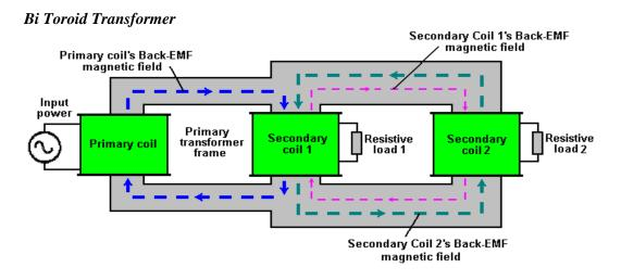
Figure 2 Bi Toroid Transformer Pulse Movements
