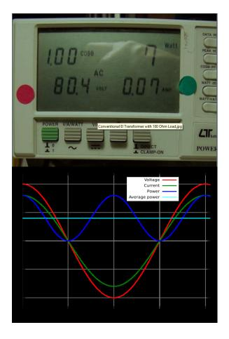
Figure 12: Conventional Transformer Sine Waves
