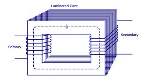
**Figure 3 Conventional Transformer**
