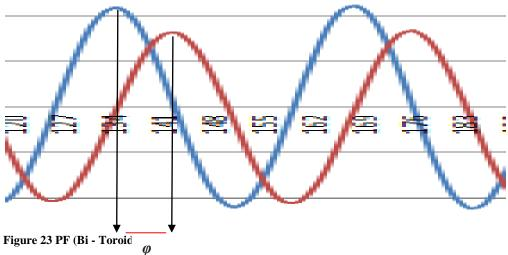
From the above graphs, it shows that the current and voltage for a Bi-Toroid transformer are almost 90° apart on the primary side. This means:
