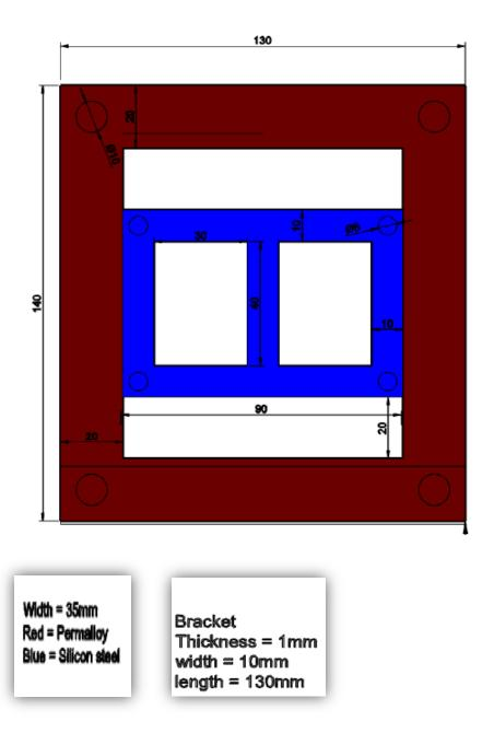
This is the proposed design of the Bi Toroid transformer. It consists of two different cores with different materials respectively. The primary core is made of silicon steel whereas the secondary coil is made of permalloy. The size of the secondary core is twice the size of the primary core; this is due to reluctance, the secondary core is less reluctant than the primary core.
