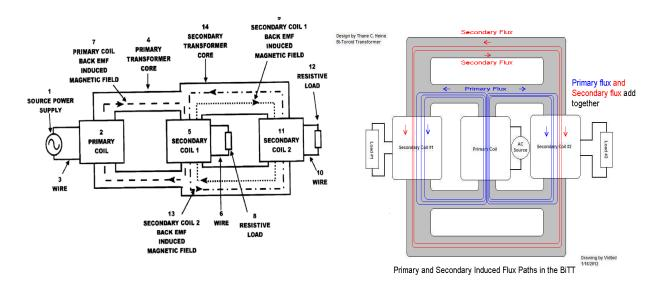
Figure 6: Bi Toroid Transformers
