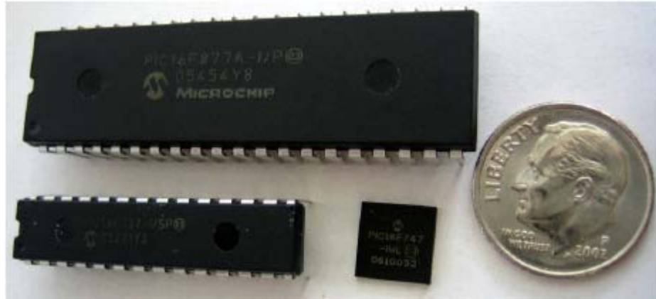
Figure 13: Size of different microcontrollers compared to a dime
