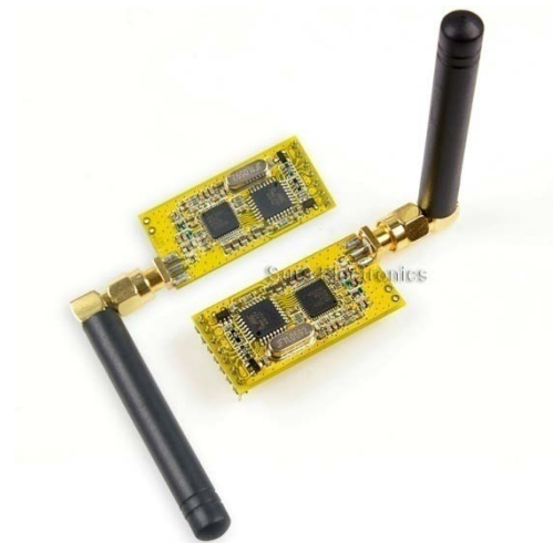
Figure 15: Wireless RF Transceiver 431-478 Mhz GFSK [12]
