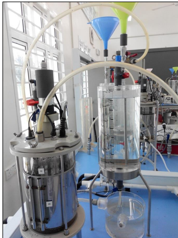
Figure 12 Gas Collection Tank (Fill with NaOH solution)
