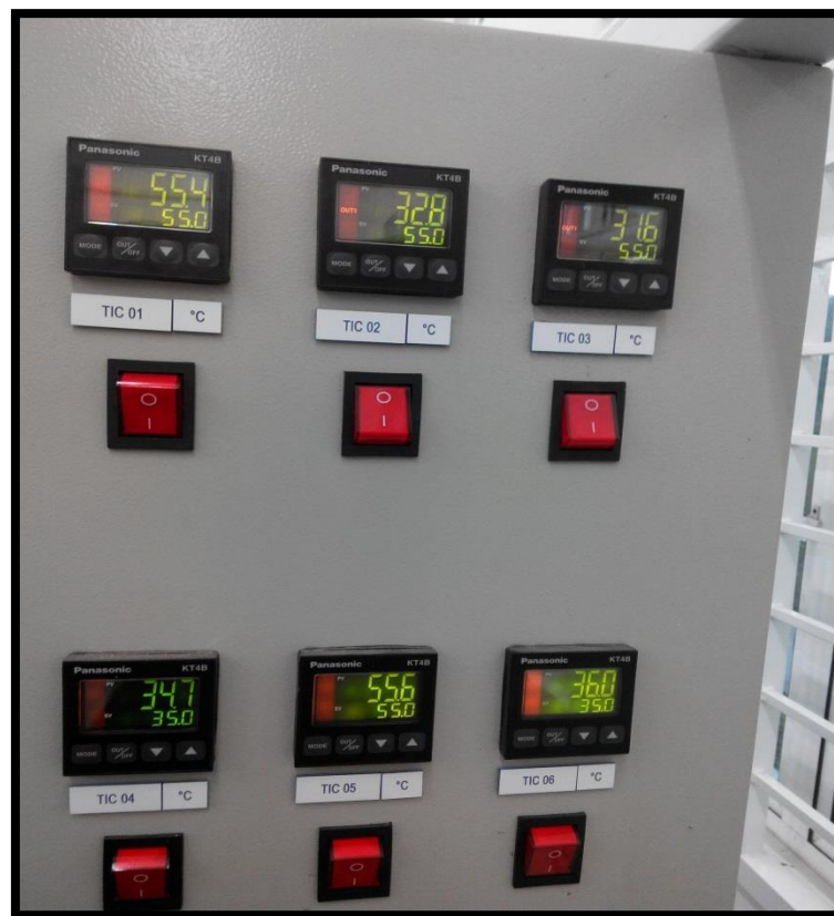
Figure 11: Meter showing the Temperature inside the reactors
