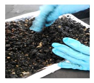
FIGURE 3.4 Mix of Petroleum Sludge with Additives
