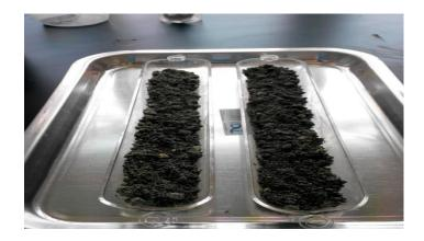
FIGURE 3.5 Treated Residue Ash
