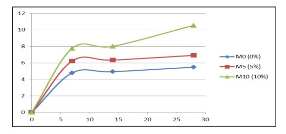
FIGURE 5.2 Compressive Strength of Mortar (MPa) in 2012 (Pakpahan et al.,2012)
