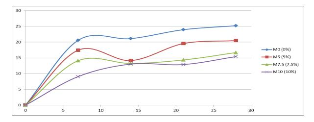
FIGURE 5.1 Compressive Strength of Mortar (MPa) in 2015 (This study)
