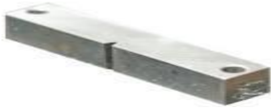
Figure 2: charpy specimen (from ASTM E23)
