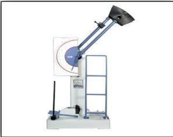
Figure 1: Impact test machine (from ASTM E23)
