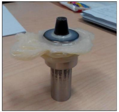
Figure 18 Accumulation of Nylon-6 material on conical pin profile
