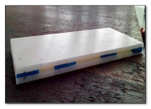
Figure 9 Nylon plate with paraffin wax slotted in the groove
