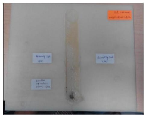
Figure 14 FSW with Straight Cylindrical Pin Profile
