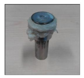
*Figure 15 Pin Profile with breakage breakage*
