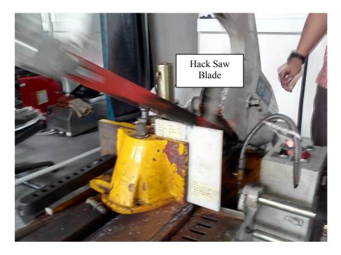
Figure 13 Hack Saw Machine during the cutting the cross section of specimens
