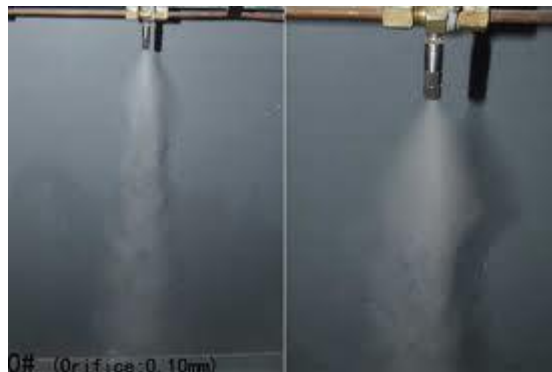
Figure 1. 1 Comparison between a single jet-like flow and a better executed mist
