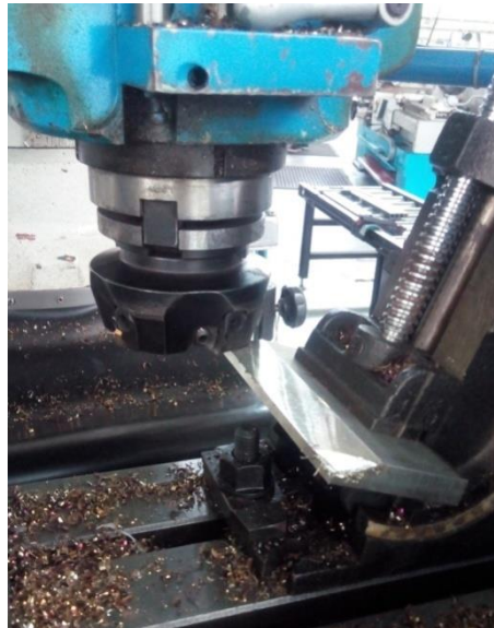
FIGURE 3.5. Milling process to create angled plate.
