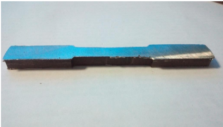
FIGURE 3.9. Tensile Specimen milled using manual milling machine.
