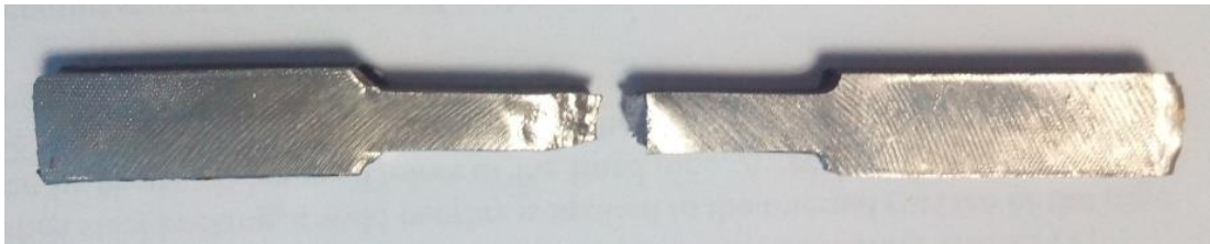
FIGURE 3.11. Sample fracture after tensile test.
