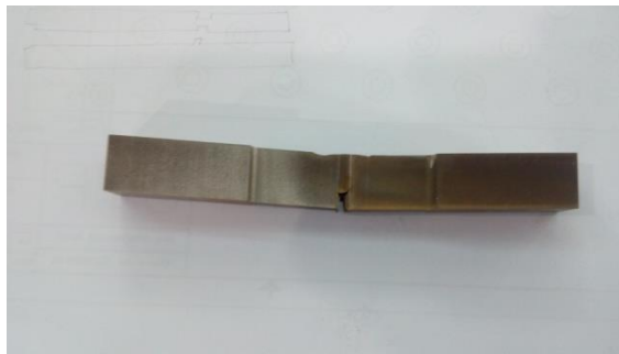
FIGURE 4.2. Incomplete penetration for 30 degree sample.
