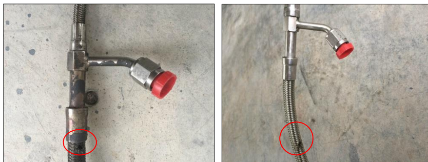
Figure 3.2: Area of failure near fittings of actual hose
