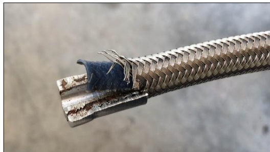
Figure 3.6: Cross section of hose fitting
