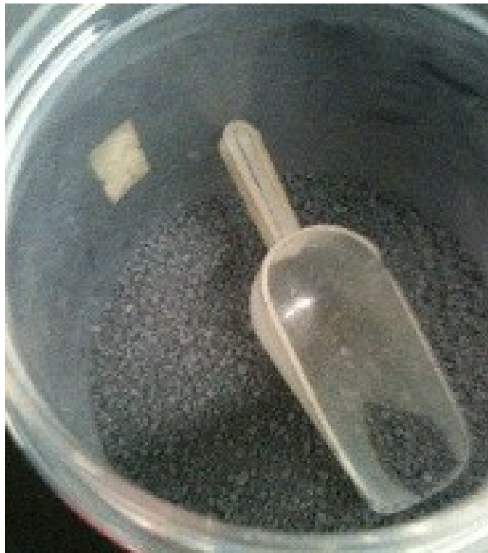
APPENDIX 8. Phenolic powder for mounting of samples
