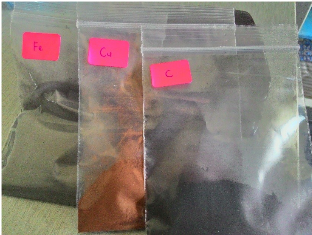
APPENDIX 1. Iron, Copper and Carbon powders before mixing
