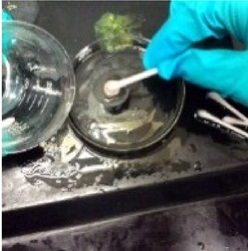
APPENDIX 13. Etching process of samples
