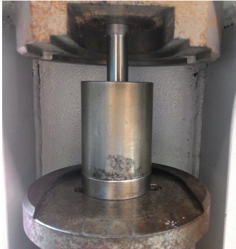
APPENDIX 3. Die in compaction process
