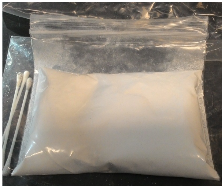
APPENDIX 4. Zinc Stearate used as die wall lubricant
