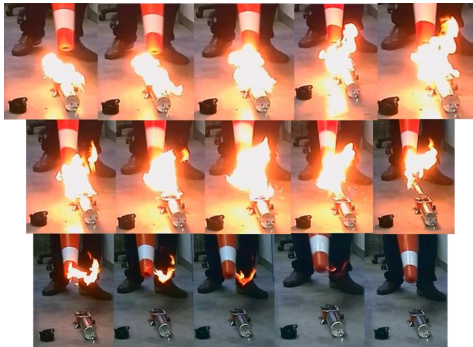
Figure 4.17: Vacuum effect of collimator by sound wave
