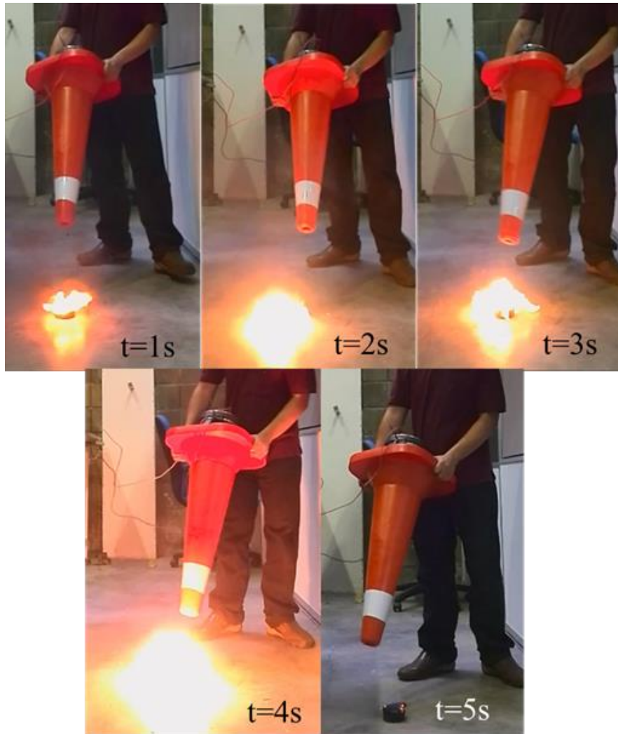
Figure 4.14: Sequence of images of solid fuel fire extinguishing
